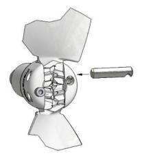
**6** Insert last pivot pin locking screw (8); turn it to engage a couple of threads; It will be tightened later in step 7;
