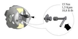
**3** Again using a straight screw driver: Bend side of tab washer up over hex on the shaft nut locking screw (6).
