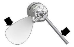
**2** Slide tab washer (5) on to shaft nut locking screw (6); screw in through hole in the shaft nut into end of shaft and tighten firmly; If using torque wrench tighten to about 15 Nm;
