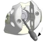
If removing prop, straighten side of tab washer to allow removal of shaft nut locking screw;
